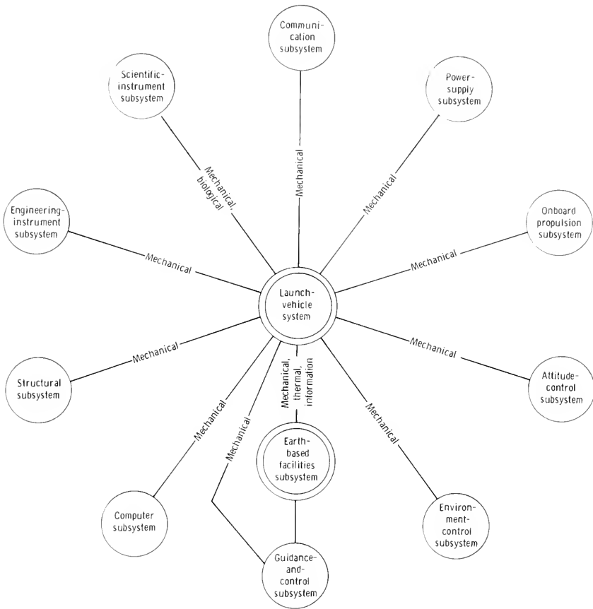
FIGURE 8-2.—Interface diagram showing the more important relationships between the launch vehicle and the rest of the satellite system.
